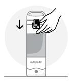
7 Once blending is complete, flip the latch down to unlock the Lid Latch.
