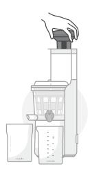
6 Drop the prepared fruits or vegetables into the feed chute and gently push the items down into the grinding assembly, using the **Food Pusher**.
