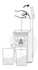
While you are juicing, you may choose to open the wide chute lid, which will open the chute to 3-inches. This will accommodate larger pieces of fruits and vegetables. When the wide chute lid is in the open position, the motor will pause and the Auger will stop rotating. After you have inserted fruits and vegetables into the large chute, close the wide chute lid to restart the motor and continue juicing.
