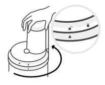
4 Twist the Juice Bowl lid counter-clockwise to unlock it, then lift to remove it from the top of the juicing jar.
