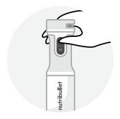
4 Press and hold either the Low speed button (I) to begin whisking operation.
