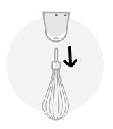
4 Separate attachment parts, if needed (Whisk–Whisk holder). The blending arm attachment is one single part.
