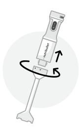
3 Detach the motor body from the blending arm or whisk attachment.
