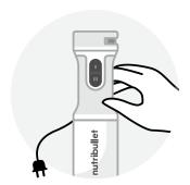
When you are done, release the Low speed button (I) and wait for whisking action to stop. Unplug the unit.
