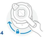
Lower the pitcher on the motor base, aligning handle on the right, and twist clockwise to lock in place. When you hear the click, it's locked and ready to blend.
