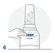
To begin blending, select a manual speed or program on the Blending Control Panel. To pause blending, press the current speed or program once, the unit will stop running and the timer will pause. To resume blending, press a manual speed or the same program.
