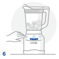
**To begin blending**, select a manual speed or program on the **Blending Control Panel**. To pause blending, press the current speed or program once, the unit will stop running and the timer will pause. **To resume blending**, press a manual speed or the same program again.
