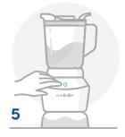
When ready, stop the appliance by pressing **POWER** (), or the function that's running, and wait for blades to stop turning.
