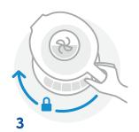
Lower the pitcher on the motor base, aligning handle on the right, and twist clockwise to lock in place. When you hear the click, it's locked and ready to blend.
