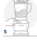
Once you reach your desired consistency, stop the appliance by pressing **POWER** <sup>(1)</sup> and wait for blades to stop turning.
