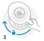
Lower the pitcher on the motor base, aligning handle on the right, and twist clockwise to lock in place. When you hear the click, it's locked and ready to blend.
