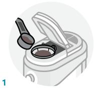
Insert the **Brew Basket + a filter**<sup>\*\*</sup> into the **Pod + Carafe Brew Area.** Use the **Coffee Ground Scoop**<sup>\*\*</sup> to measure the appropriate amount of coffee grounds into your filter.<sup>\*\*</sup>
