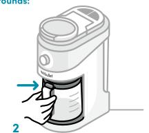
Place the **Carafe** onto the heat plate.
