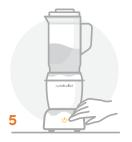
When ready, stop the appliance by pressing **POWER**  $\bigcirc$ , or the function that's running, and wait for blades to stop turning.
