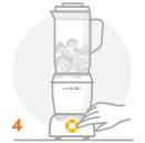
Press **POWER** <sup>()</sup>, then select a speed or the Extract program on the blending control panel.
