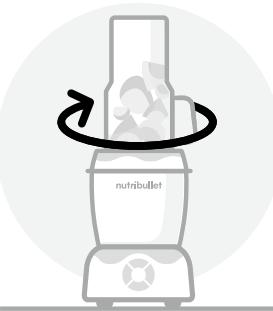
Turn the cup upside down and place it onto the motor base, gently turning the cup clockwise to lock into the motor base.
