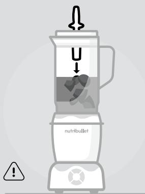
**CAUTION:** Do not use any apparatus or utensil other than the tamper to push ingredients toward the blade. The tamper is specifically designed not to come in contact with the blade. Spatulas, spoons and other tools are long enough to reach the blade, which may result in damage to the machine, damage to property, and possible injury.
